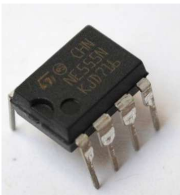
8 Pin IC (Note notch on left side of chip indicating the end with pin one.)
